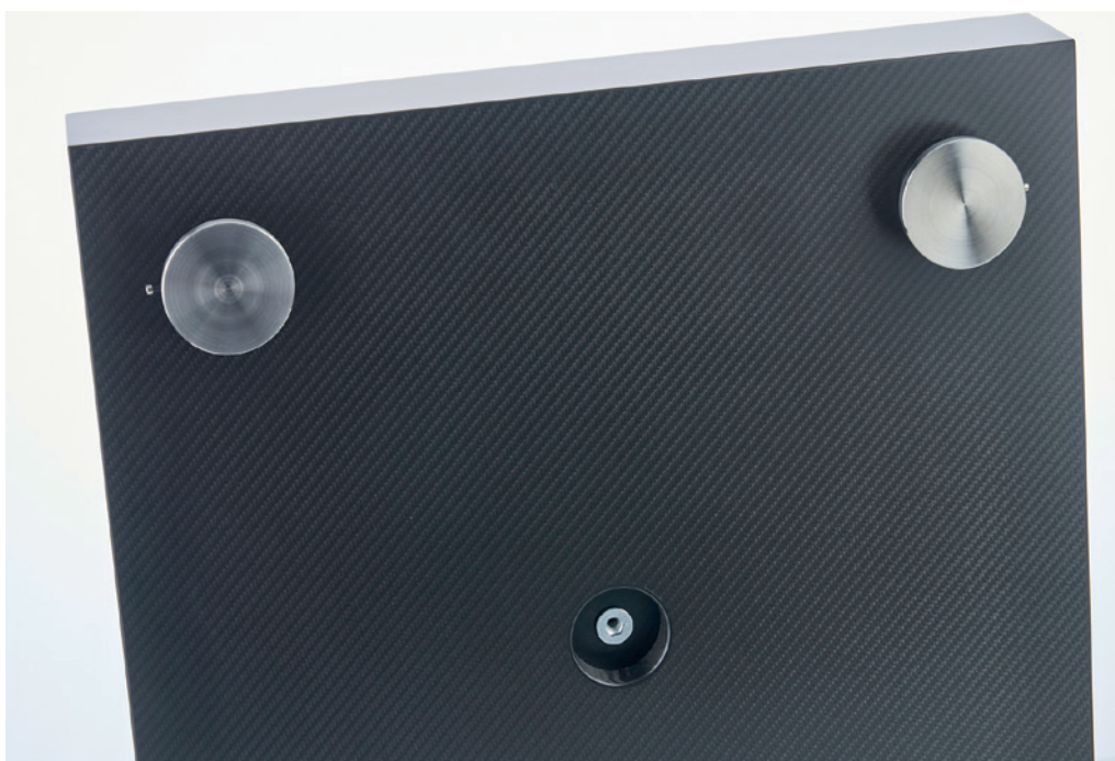
The underside of the tested isolation base with two of the four feet. Another can be screwed into the mount in the middle
